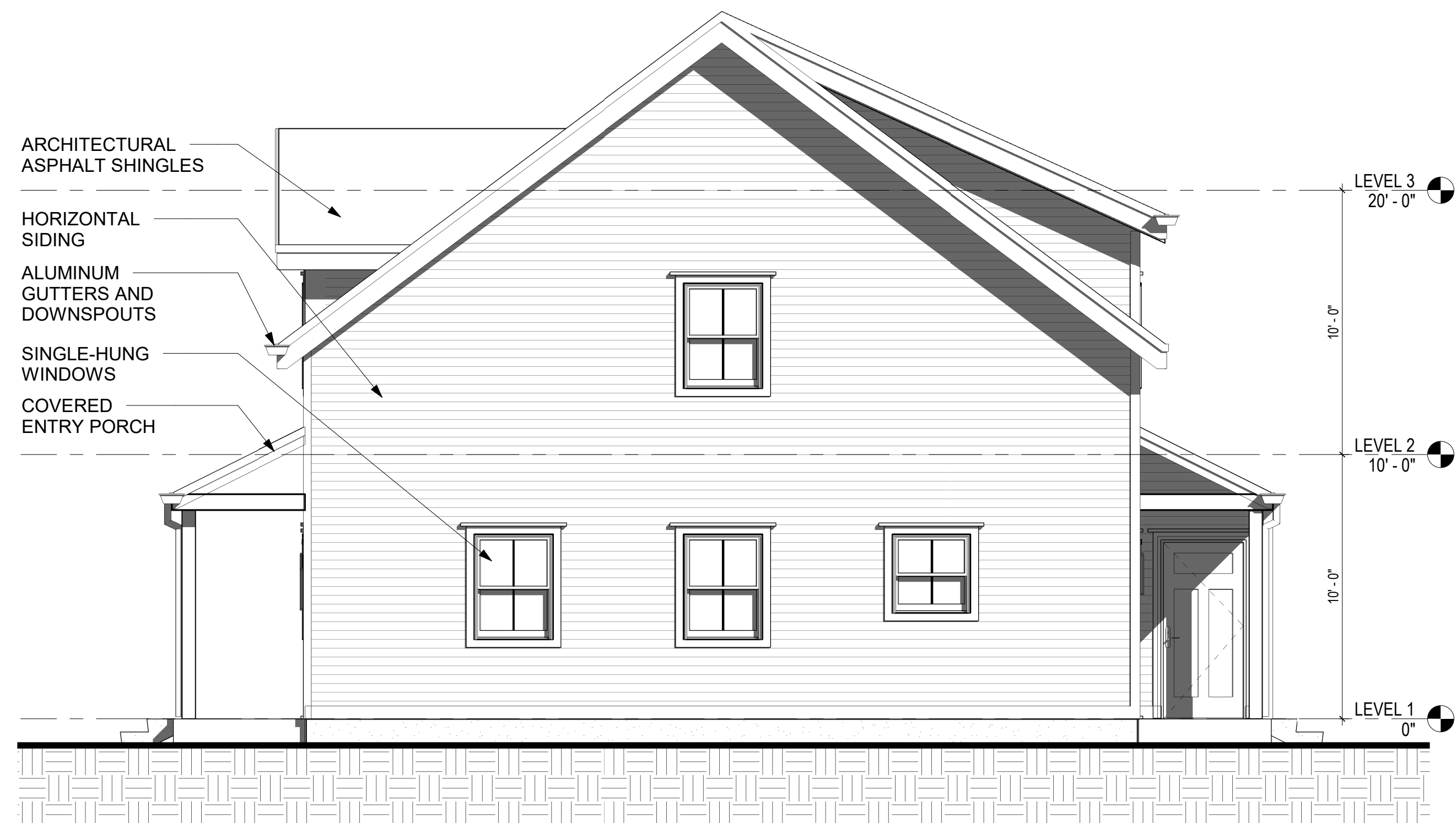
2 RIGHT ELEVATION - BUILDING 1 & 3 A3.0A 1/4" = 1'-0"
