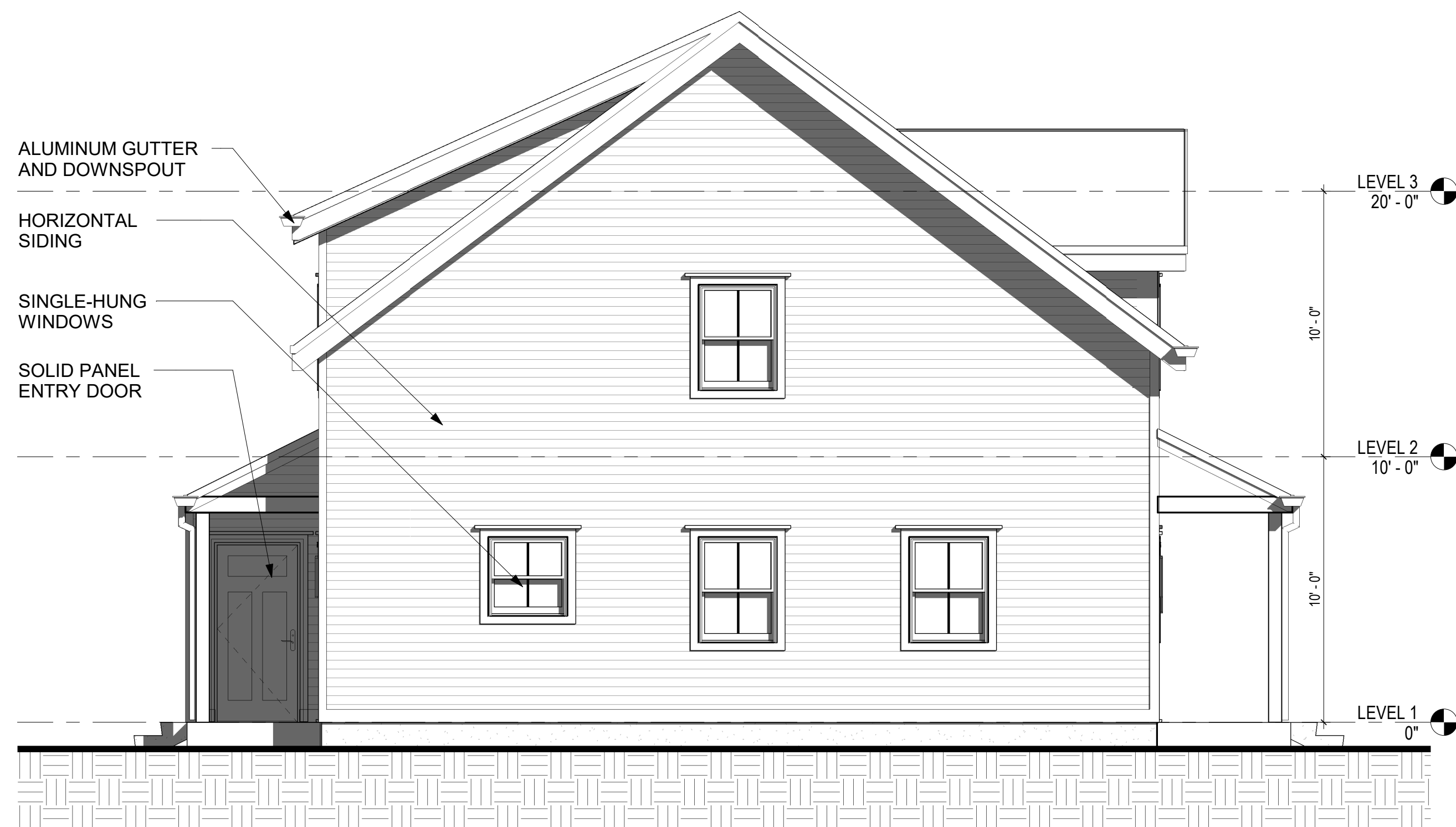
4 LEFT ELEVATION - BUILDING 1 & 3 A3.0A 1/4" = 1'-0"
