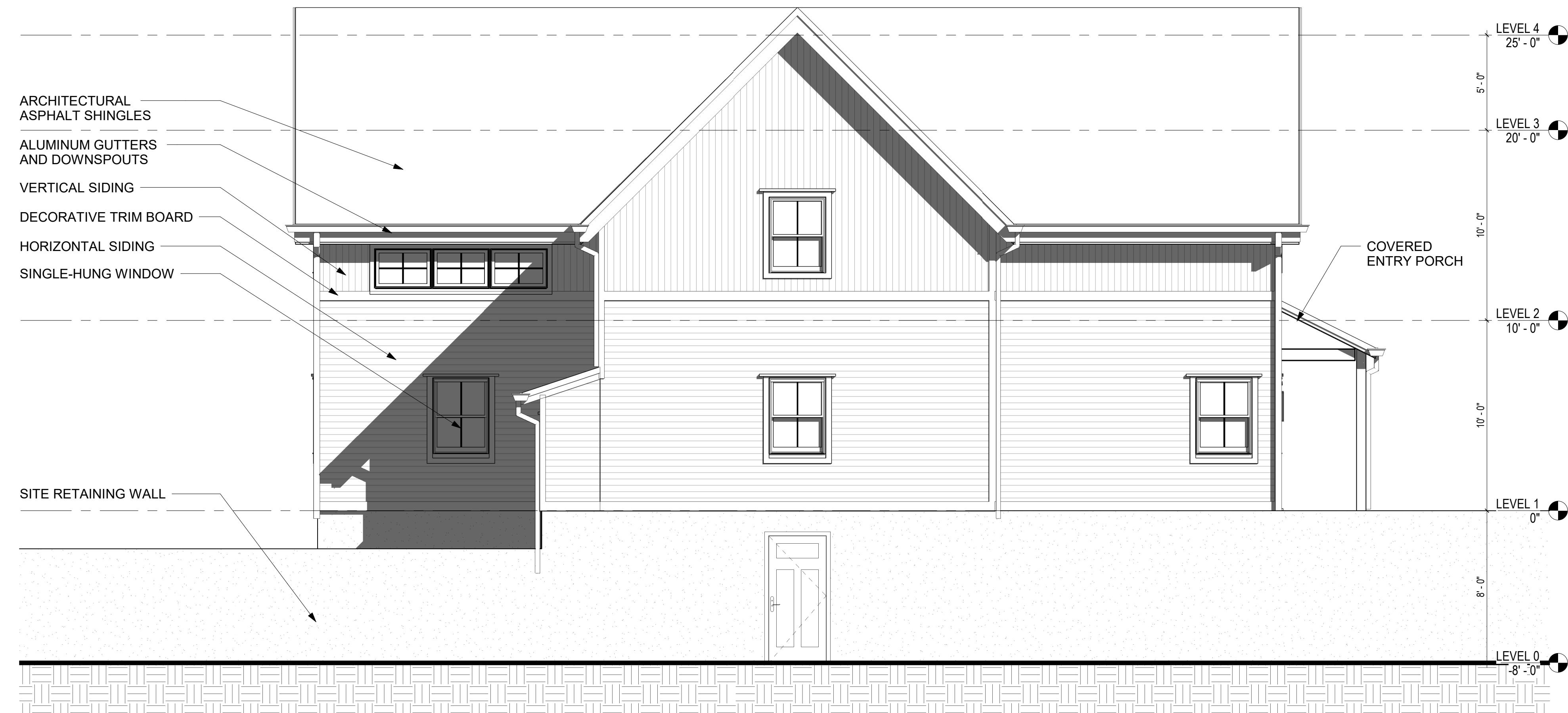
1 BACK ELEVATION - BUILDING 4 A3.0D 1/4" = 1'-0"
