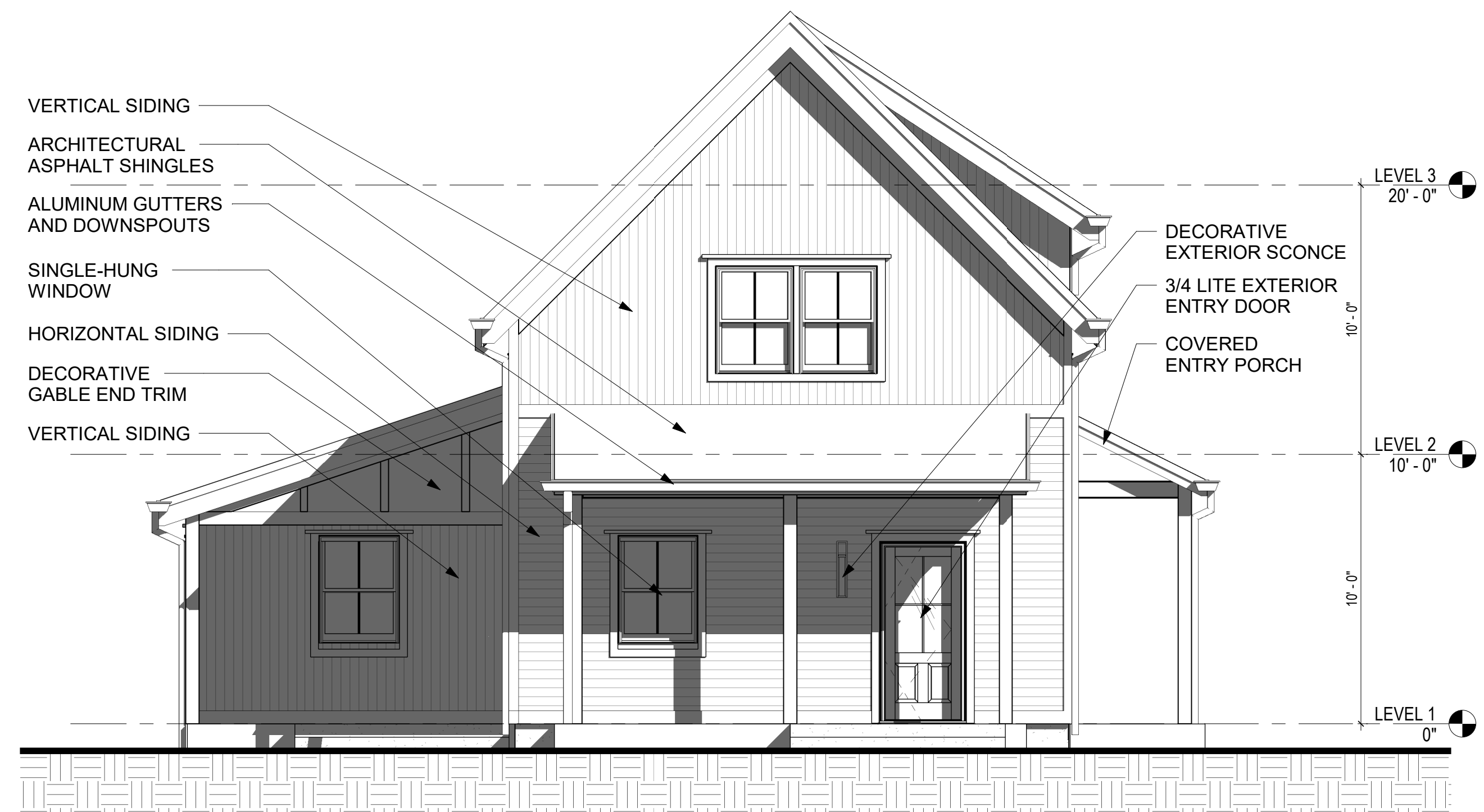
1 FRONT ELEVATION - BUILDING 6 A3.1E 1/4" = 1'-0"
