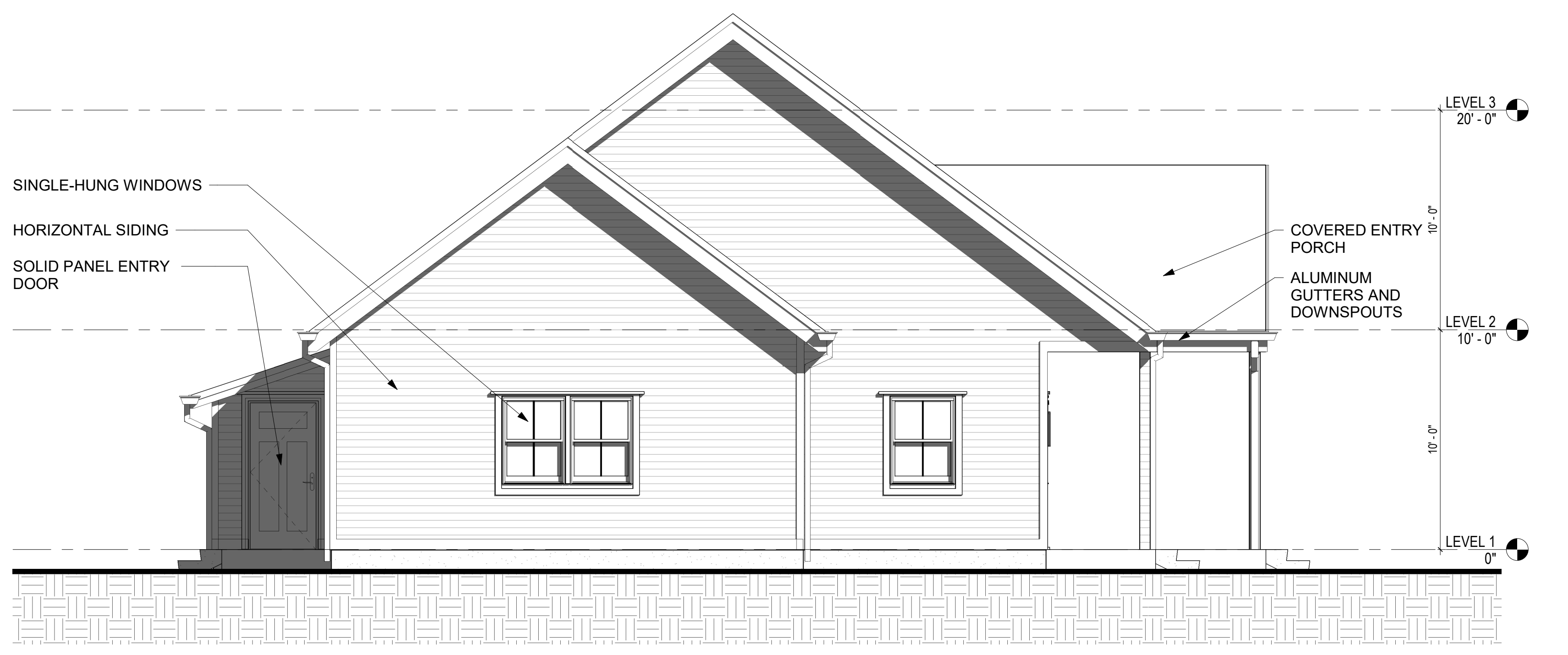
1 A3.3B LEFT ELEVATION - BUILDING 9 1/4" = 1'-0"
