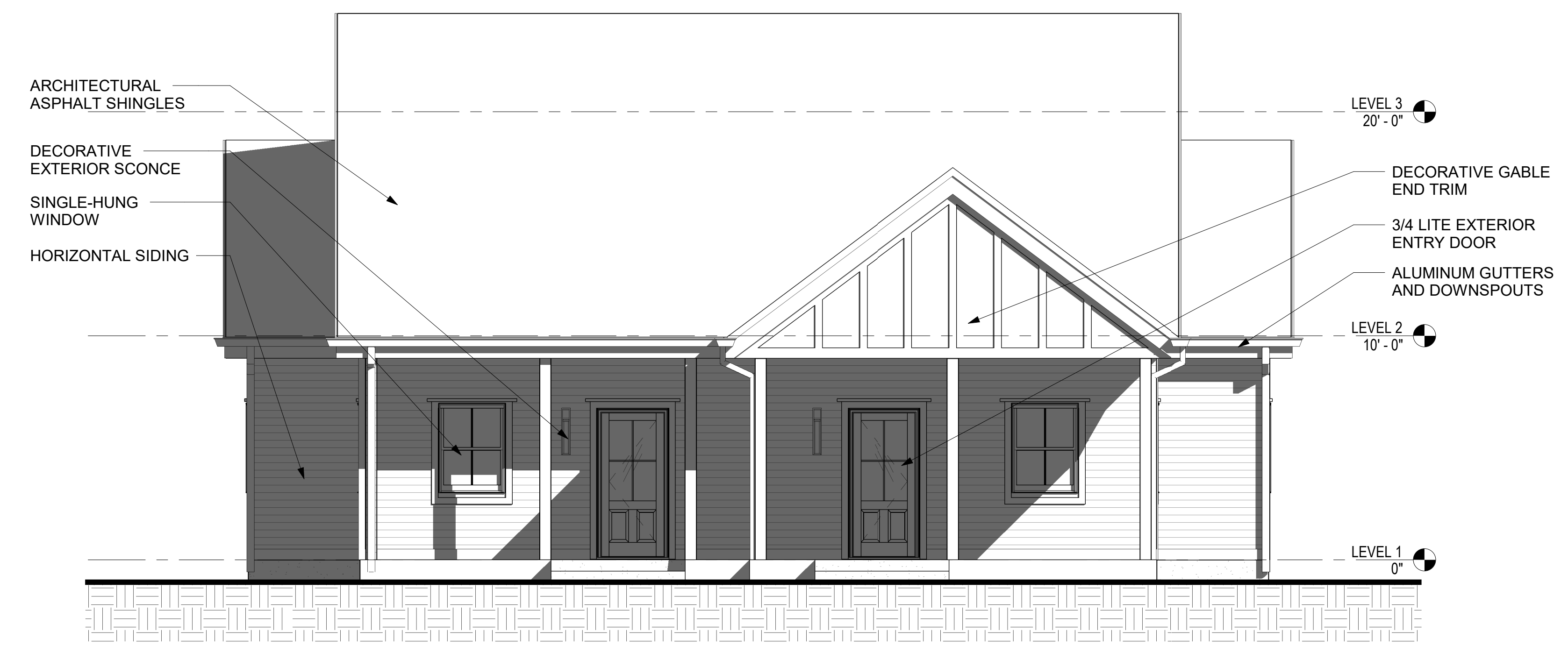
2 FRONT ELEVATION - BUILDING 9 A3.2B 1/4" = 1'-0"
