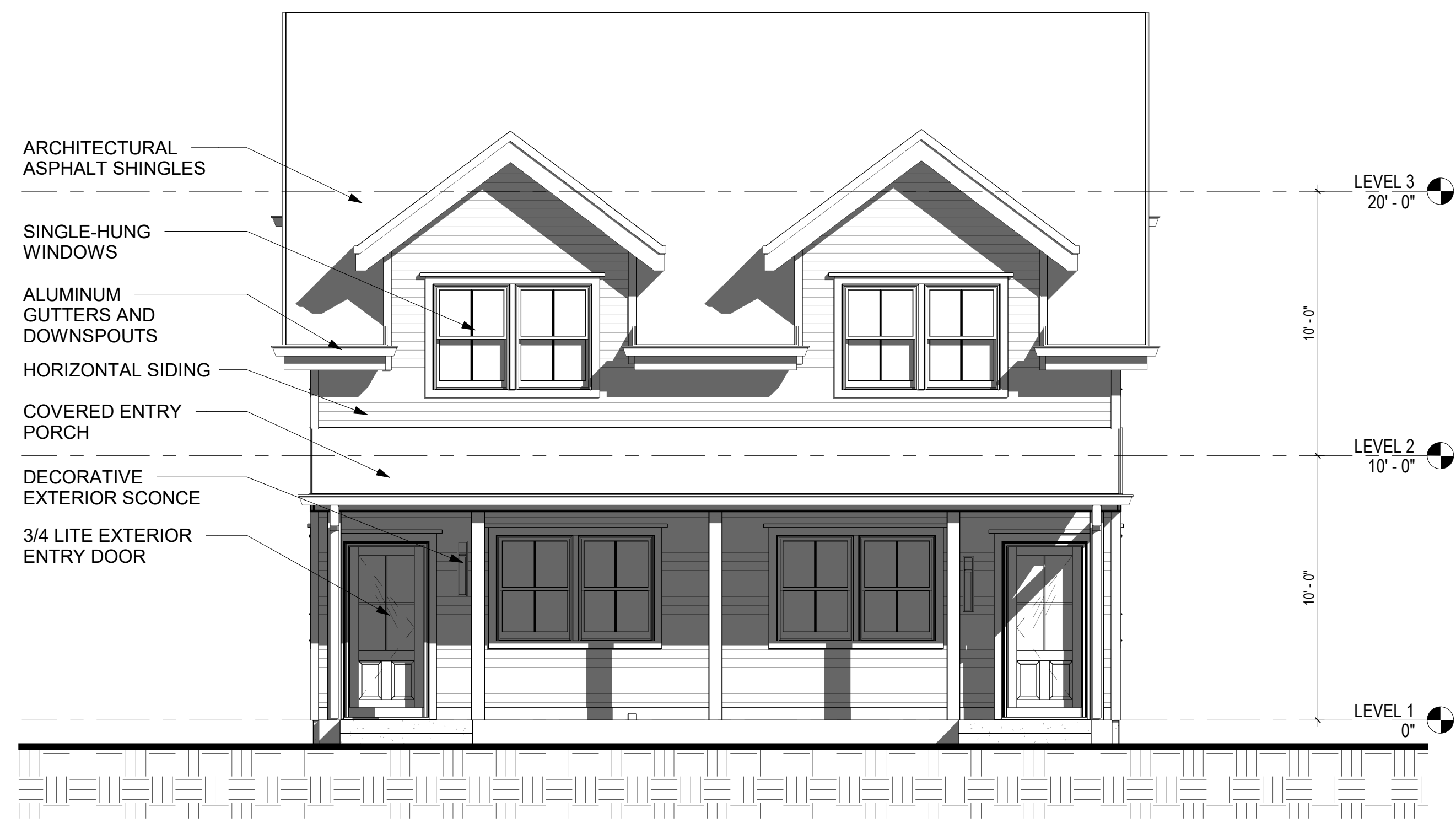
1 FRONT ELEVATION - BUILDING 1 & 3 A3.0A 1/4" = 1'-0"
