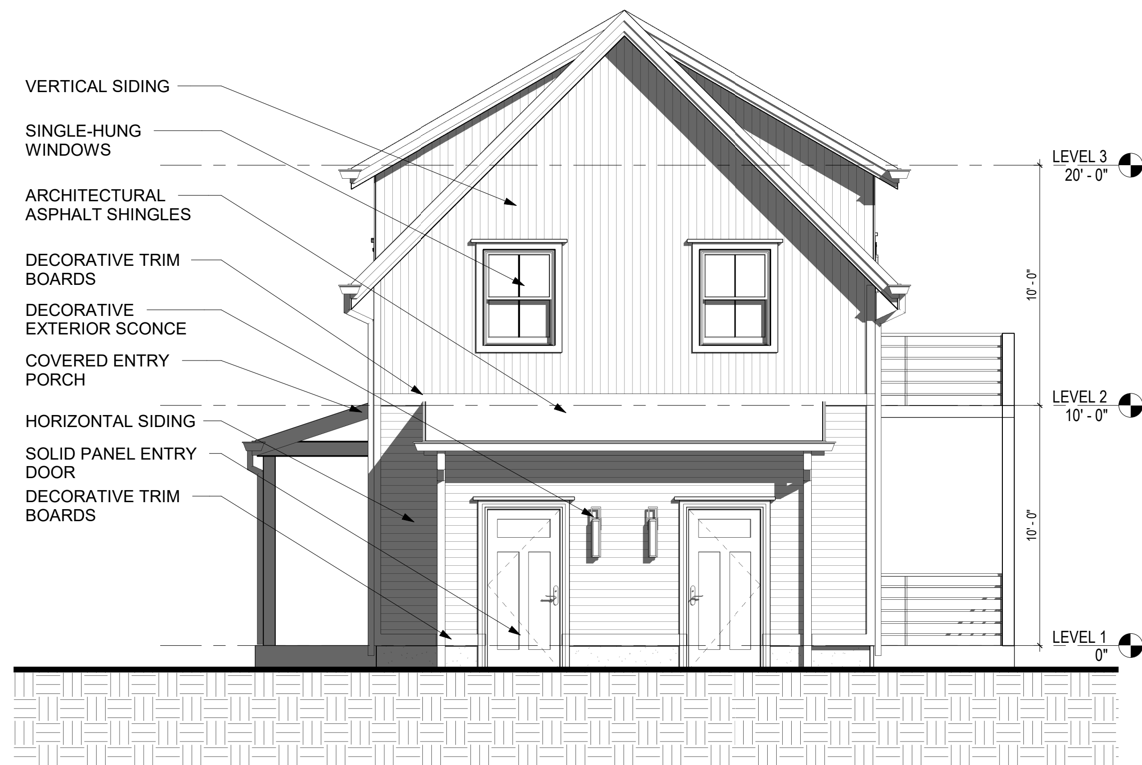
2 RIGHT ELEVATION - BUILDING 2 A3.1C 1/4" = 1'-0"
