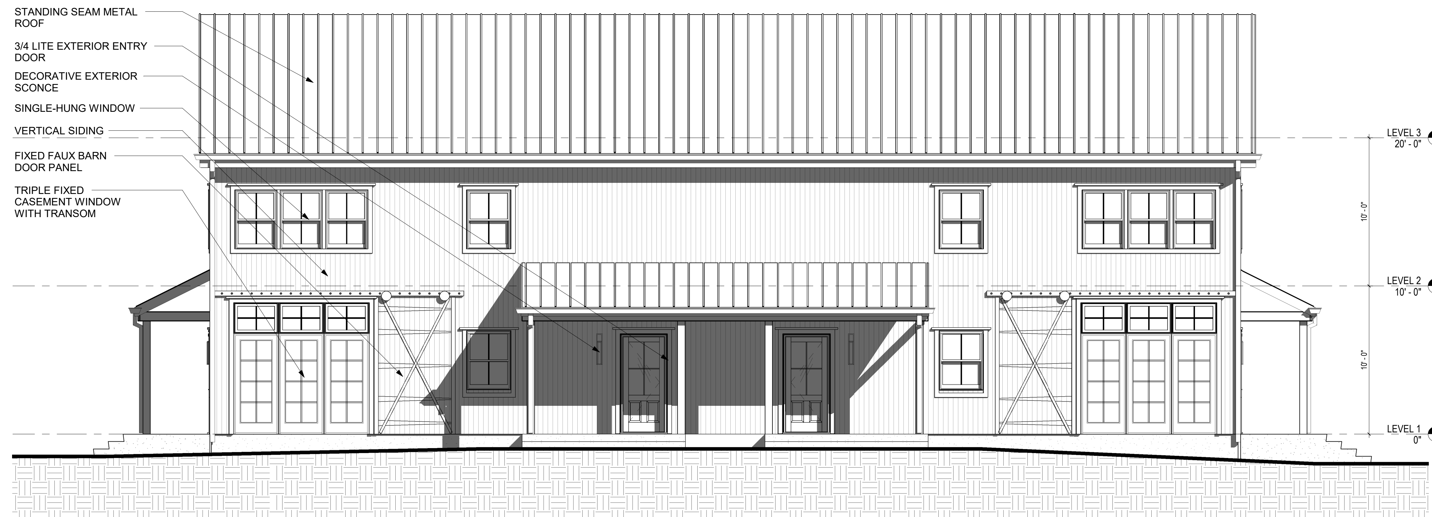
1 FRONT ELEVATION - BUILDING 7 A3.0F 1/4" = 1'-0"
