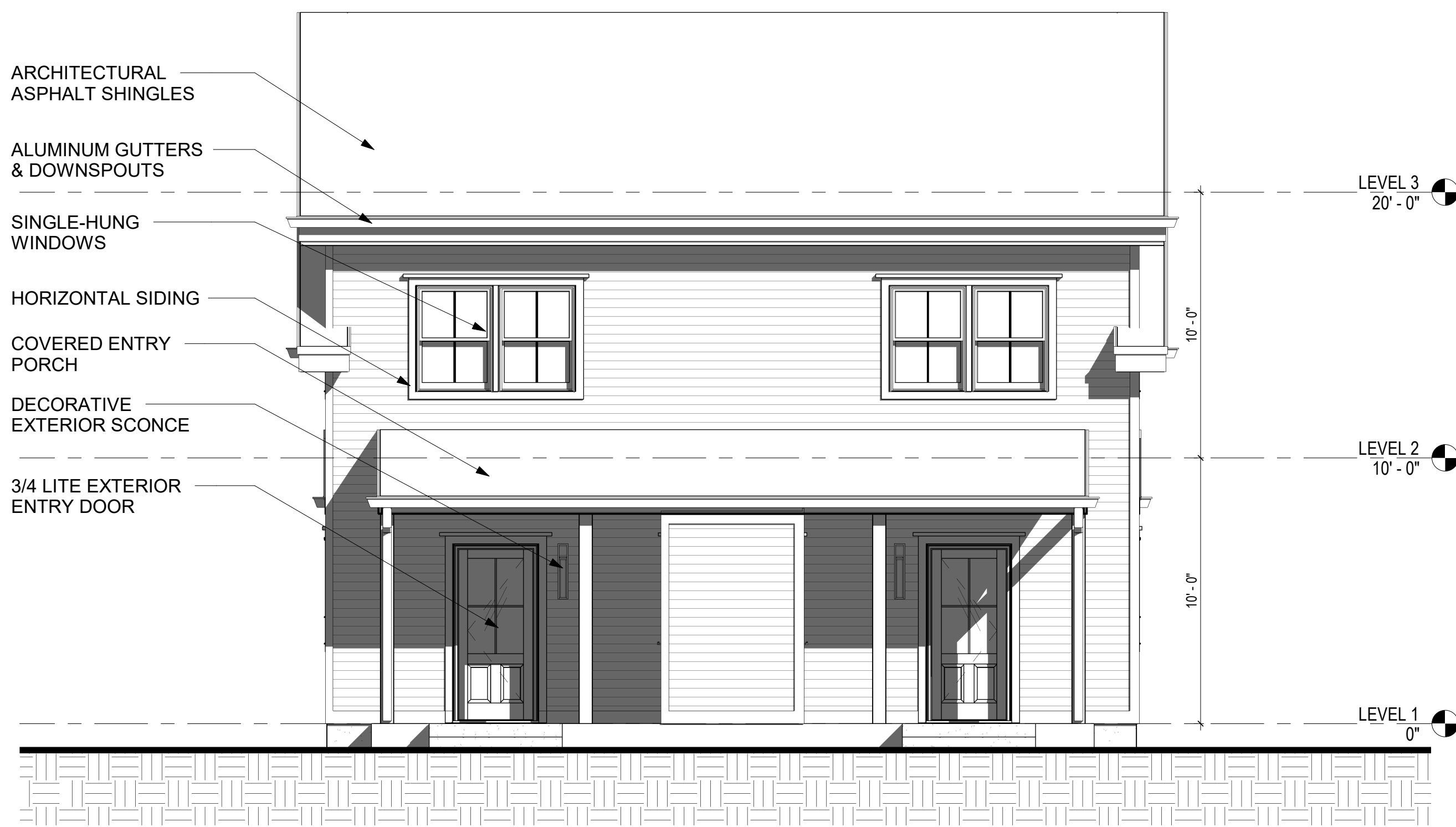
3 BACK ELEVATION - BUILDING 1 & 3 A3.0A 1/4" = 1'-0"
