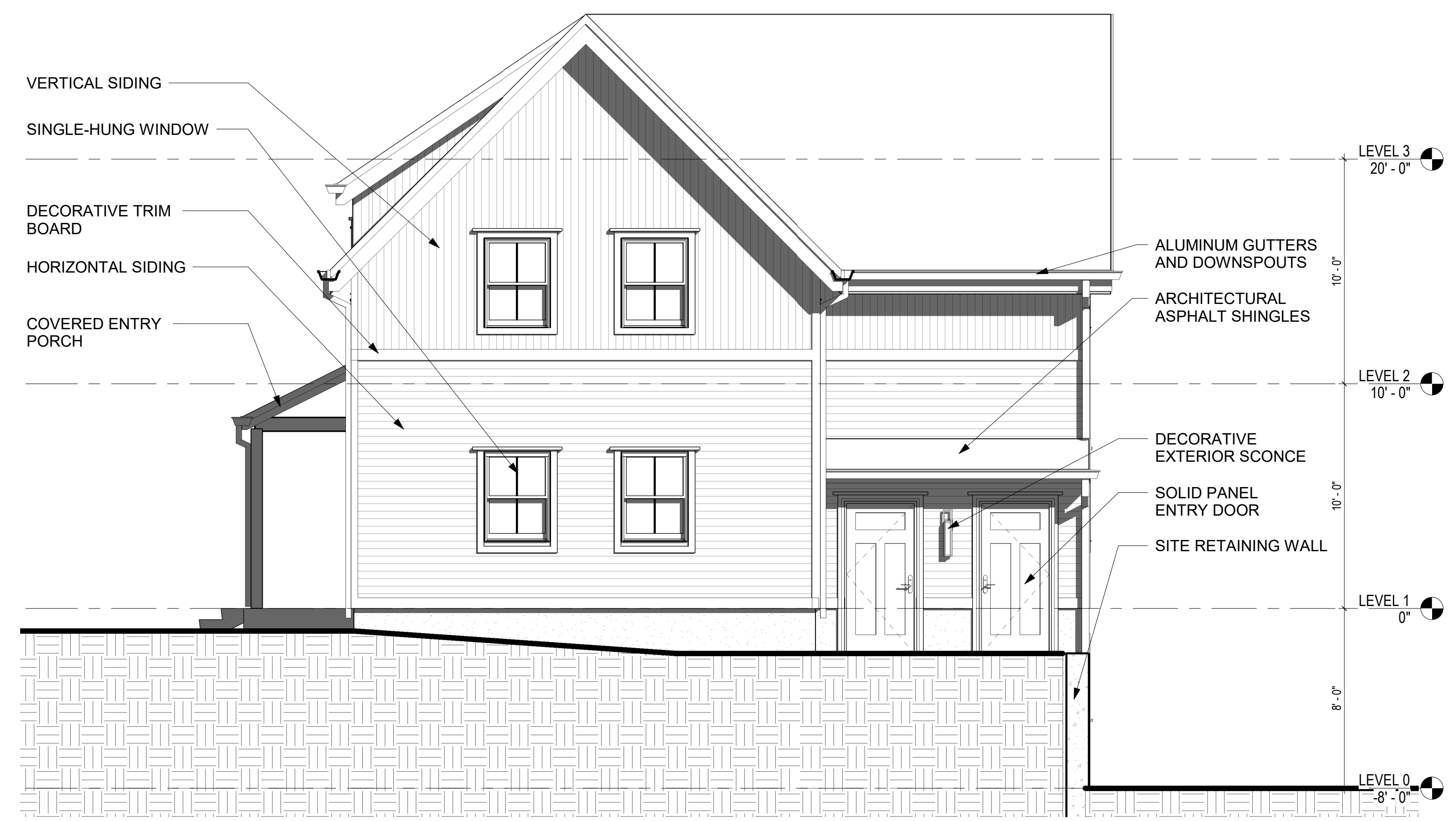
1 RIGHT ELEVATION - BUILDING 4 A3.1D 1/4" = 1'-0"
