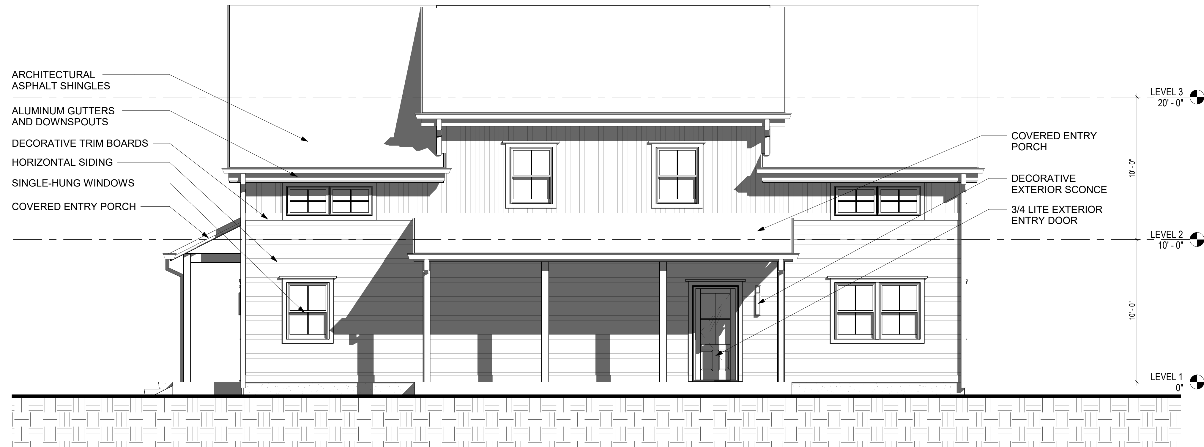
4 RIGHT ELEVATION - BUILDING 6 A3.0E 1/4" = 1'-0"
