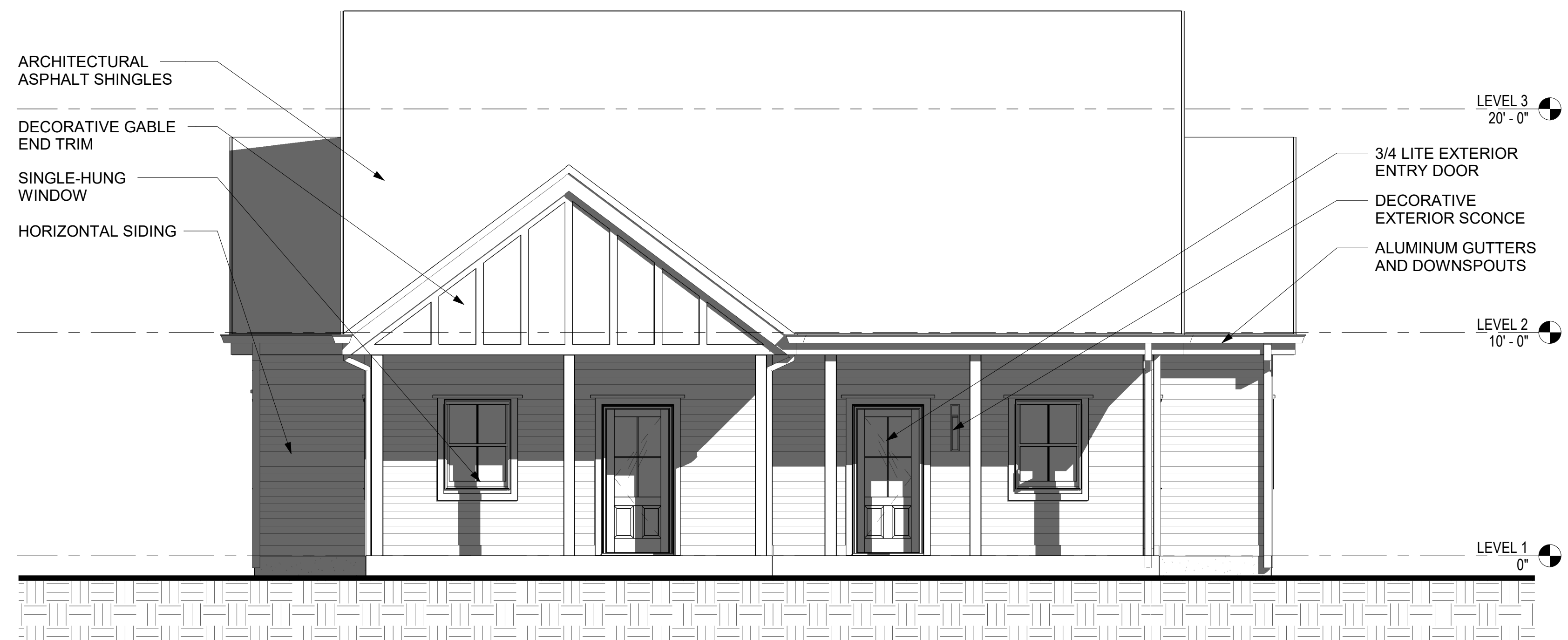
2 FRONT ELEVATION - BUILDING 5 A3.0B 1/4" = 1'-0"
