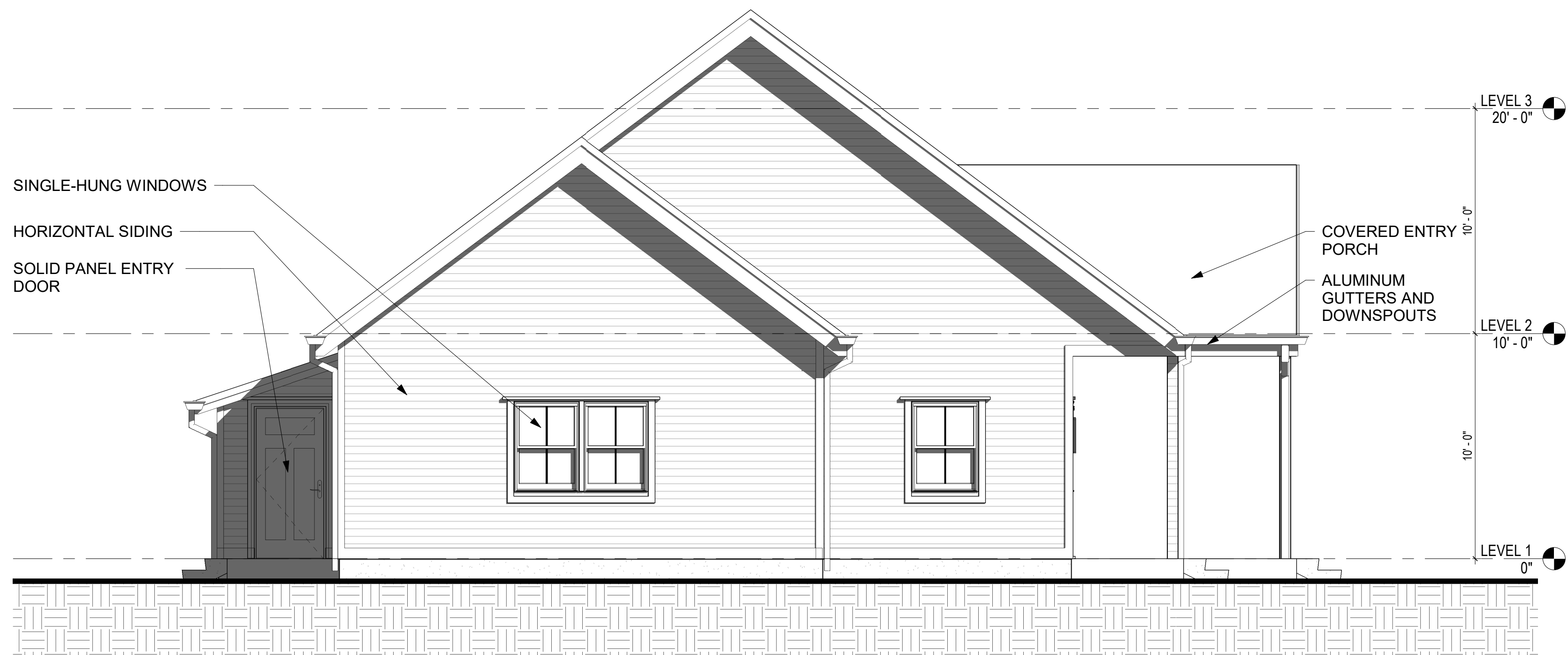
1 LEFT ELEVATION - BUILDING 9
