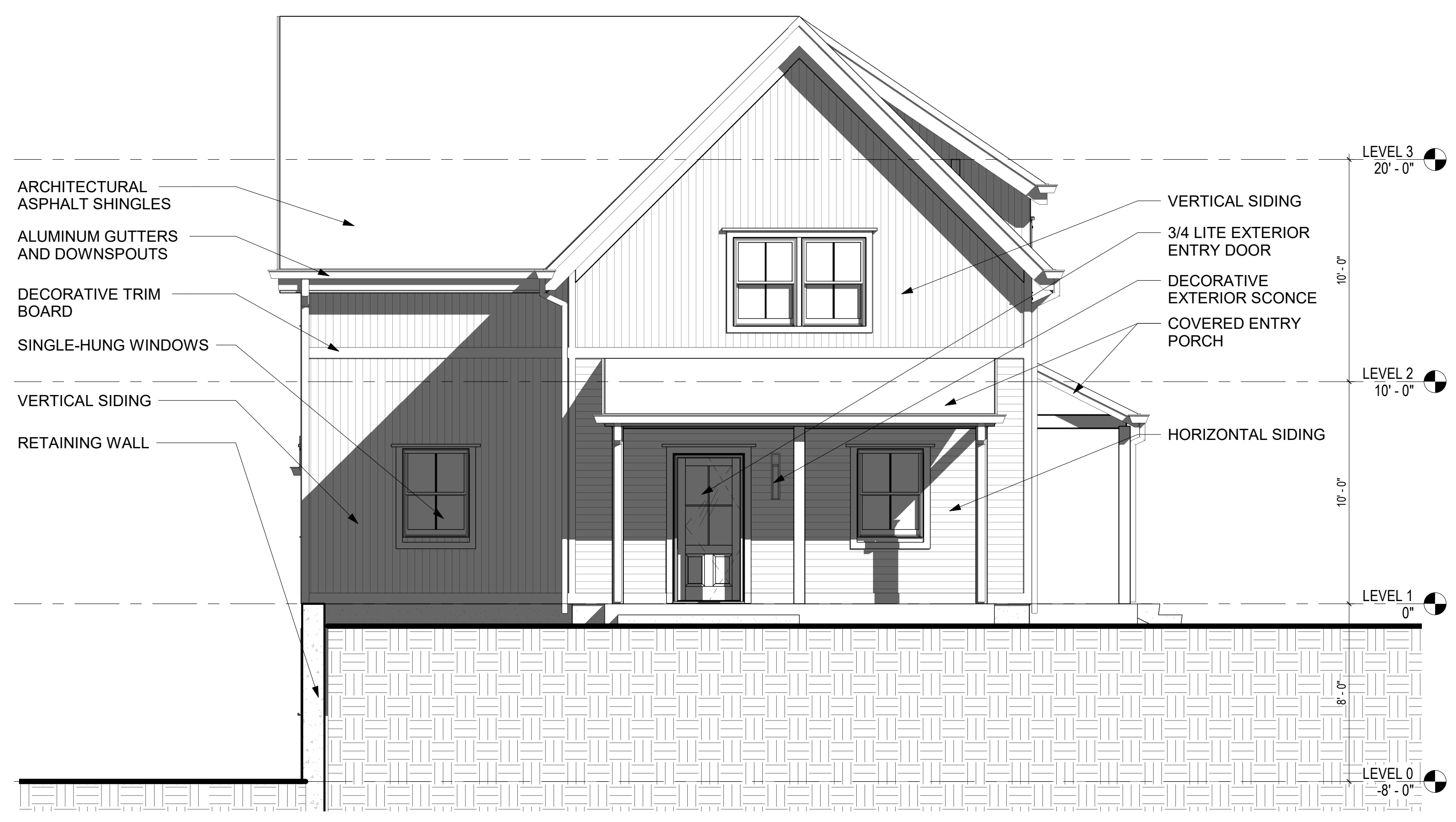
2 LEFT ELEVATION - BUILDING 4 A3.1D 1/4" = 1'-0"
