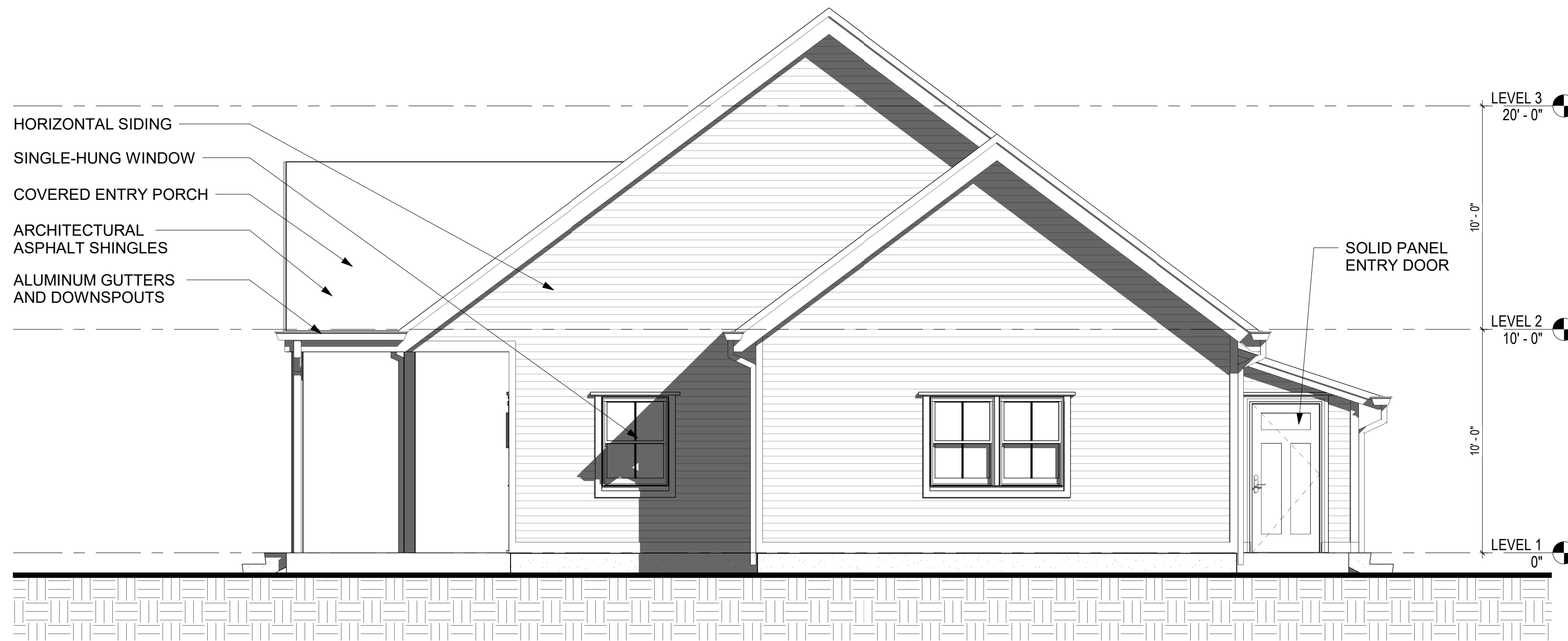
2 RIGHT ELEVATION - BUILDING 9
