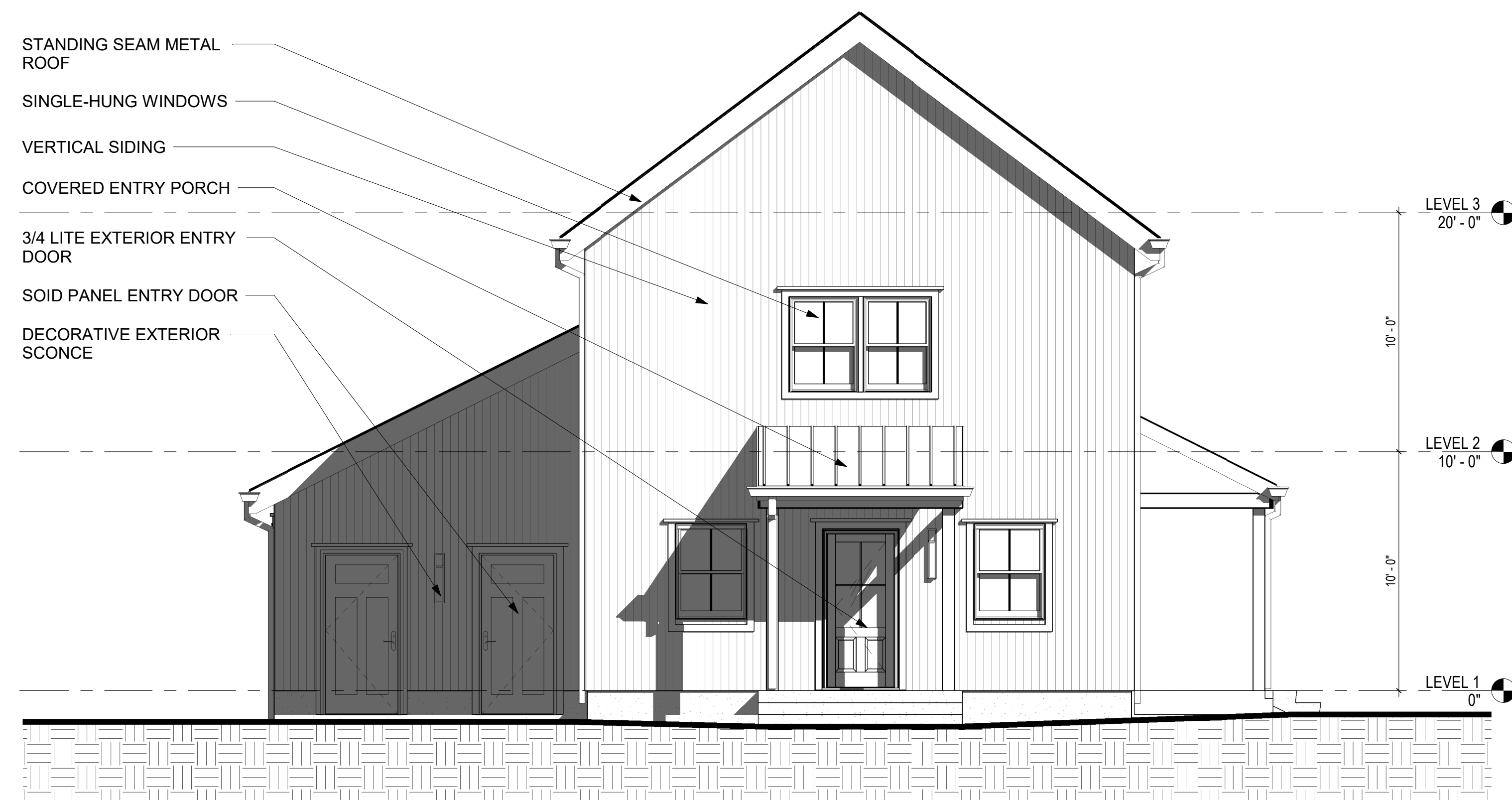
1 LEFT ELEVATION - BUILDING 7 A3.1F 1/4" = 1'-0"
