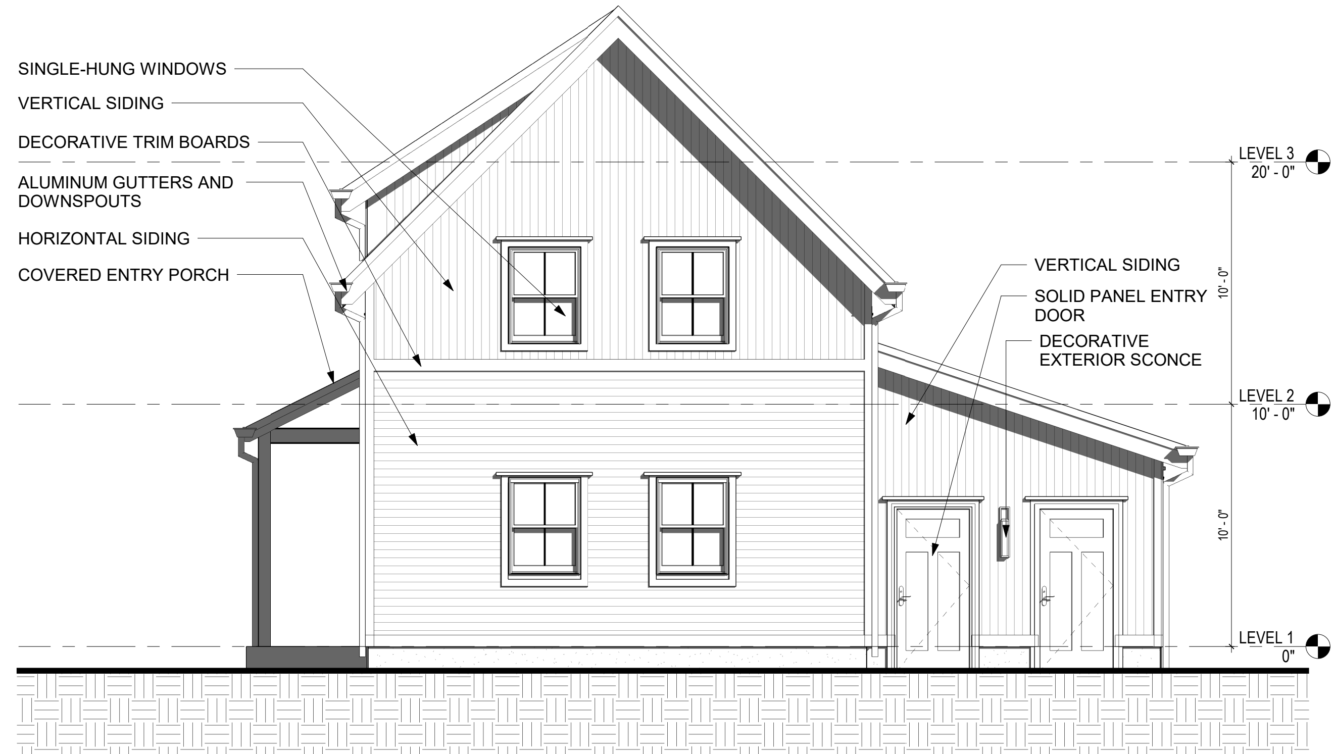
2 BACK ELEVATION - BUILDING 6 A3.1E 1/4" = 1'-0"
