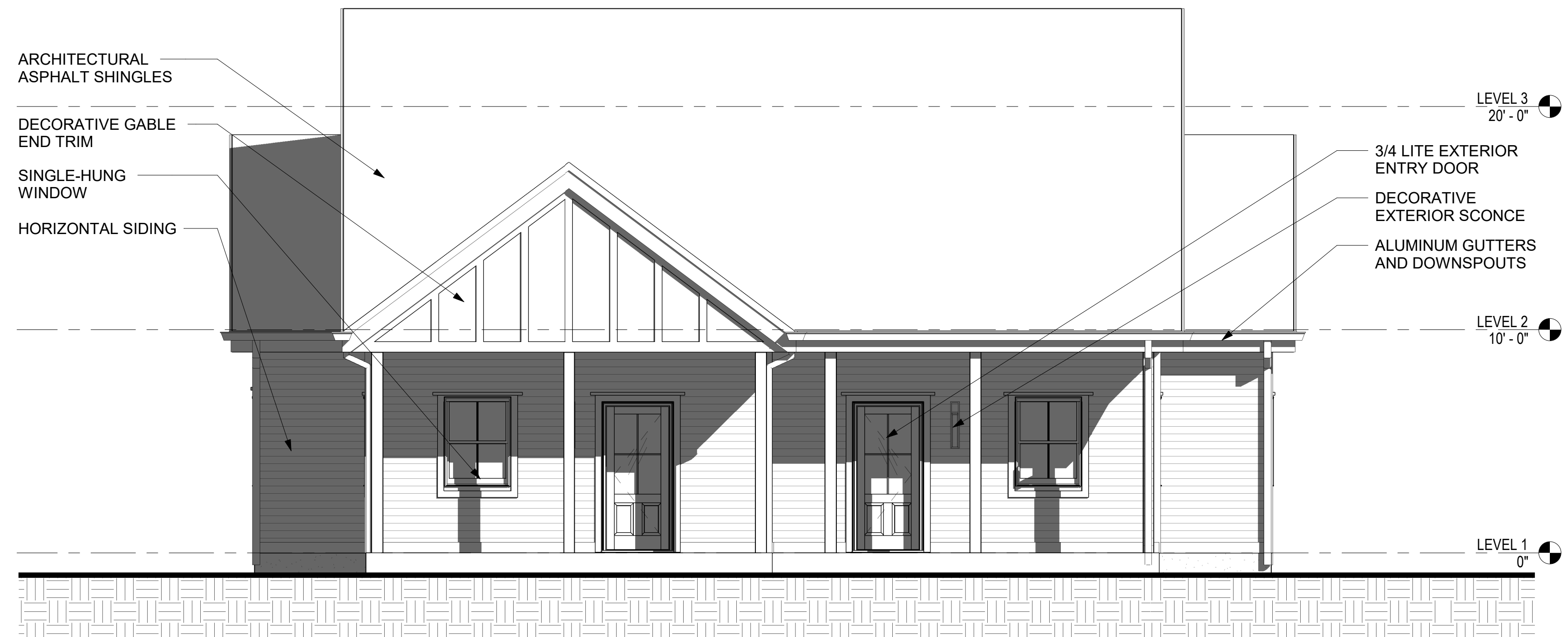
2 FRONT ELEVATION - BUILDING 5 A3.0B 1/4" = 1'-0"
