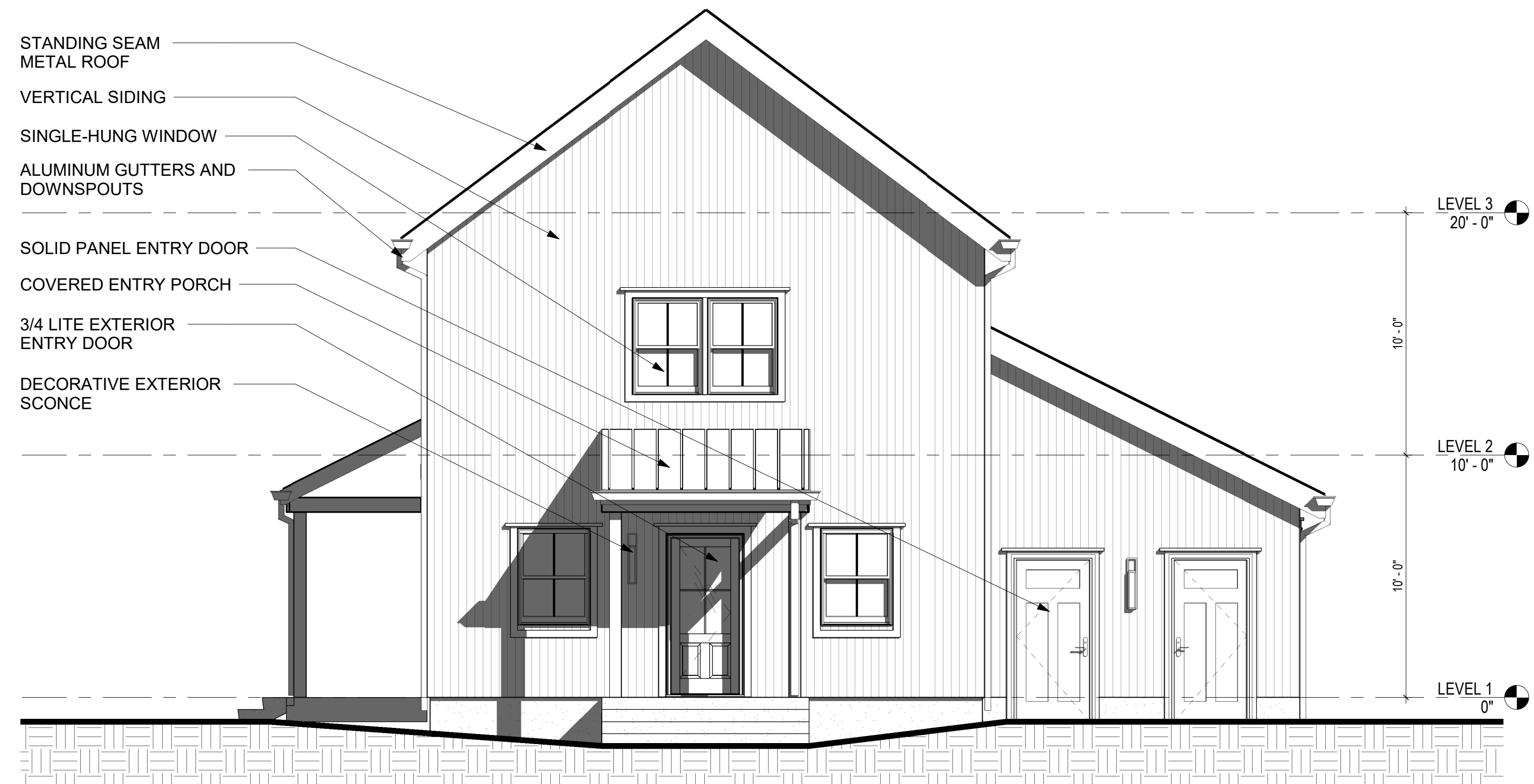
2 RIGHT ELEVATION - BUILDING 7 A3.1F 1/4" = 1'-0"
