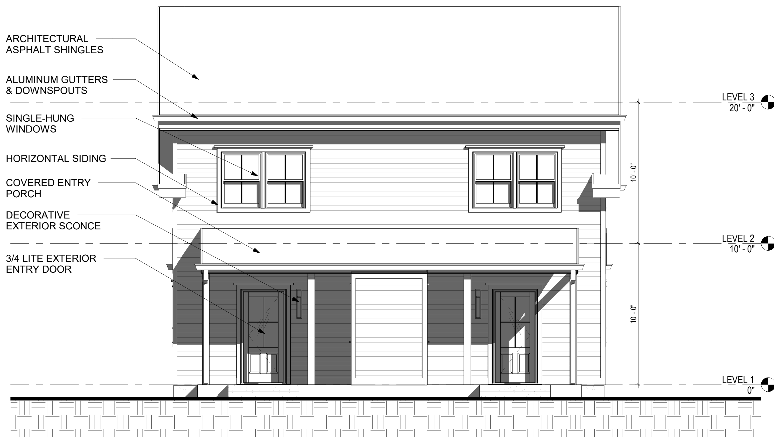
3 BACK ELEVATION - BUILDING 1 & 3 A3.0A 1/4" = 1'-0"
