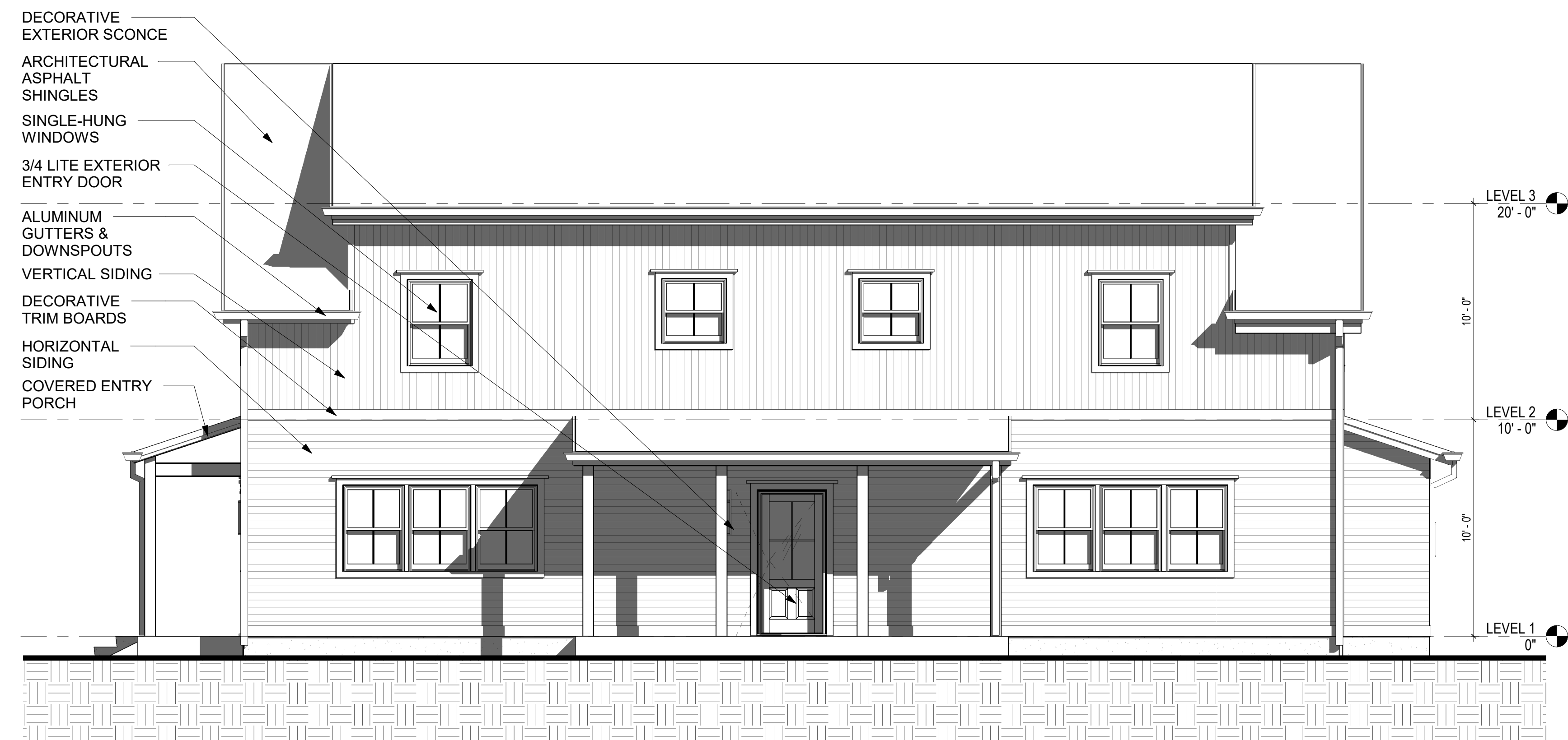
1 FRONT ELEVATION - BUILDING 2 A3.0C 1/4" = 1'-0"
