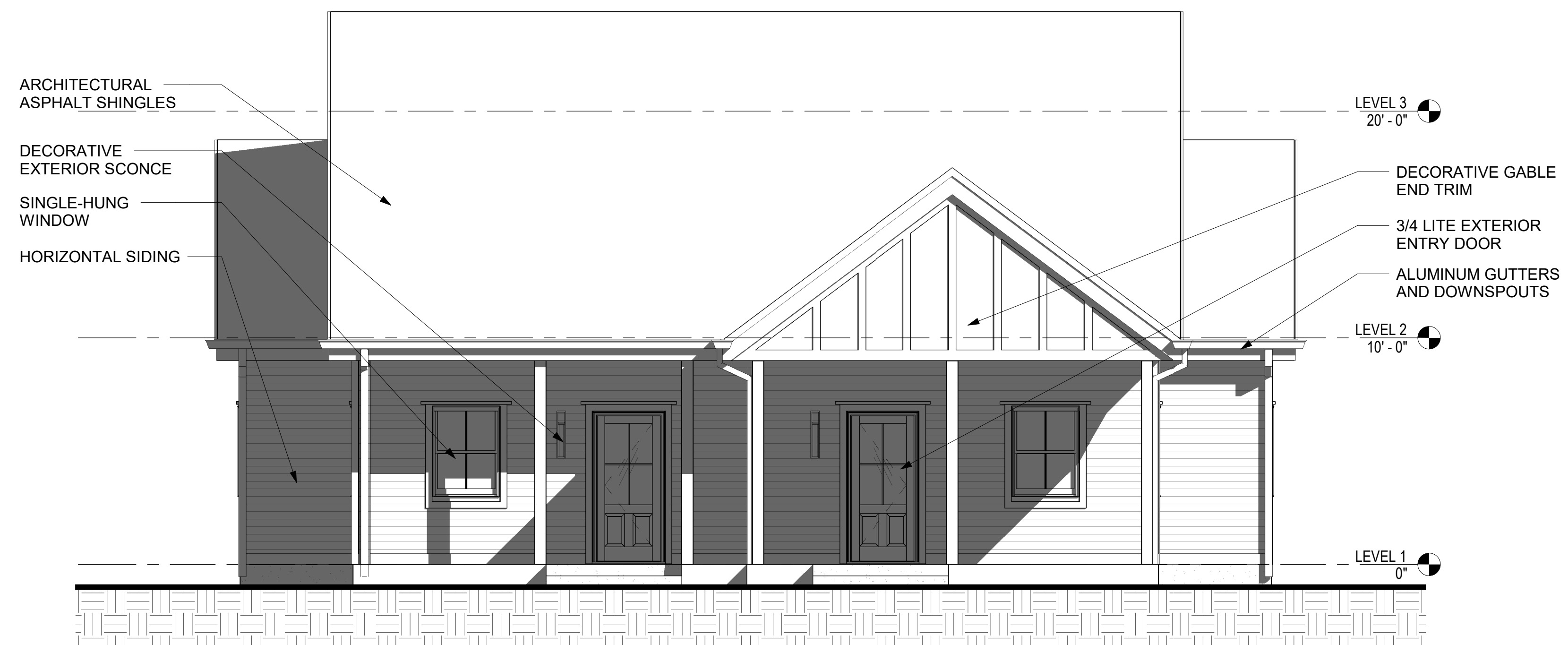
2 FRONT ELEVATION - BUILDING 9 A3.2B 1/4" = 1'-0"
