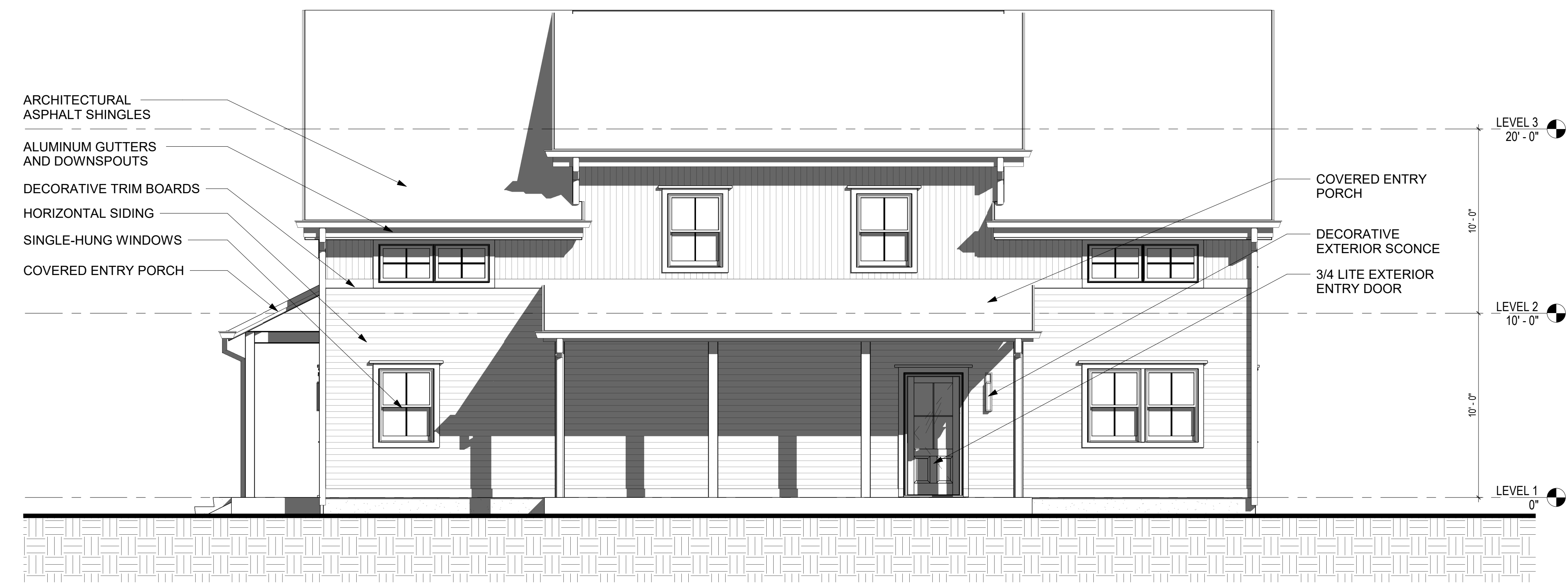
4 RIGHT ELEVATION - BUILDING 6 A3.0E 1/4" = 1'-0"
