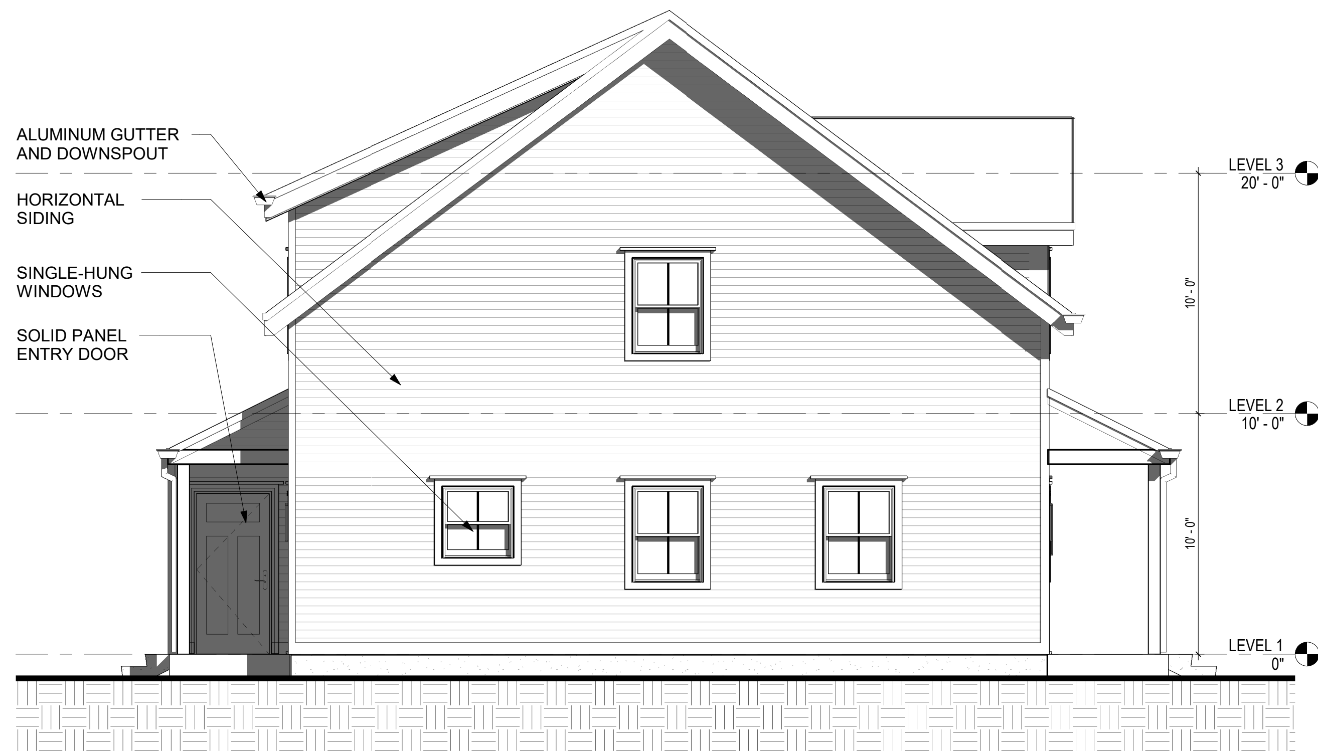
4 LEFT ELEVATION - BUILDING 1 & 3 A3.0A 1/4" = 1'-0"
