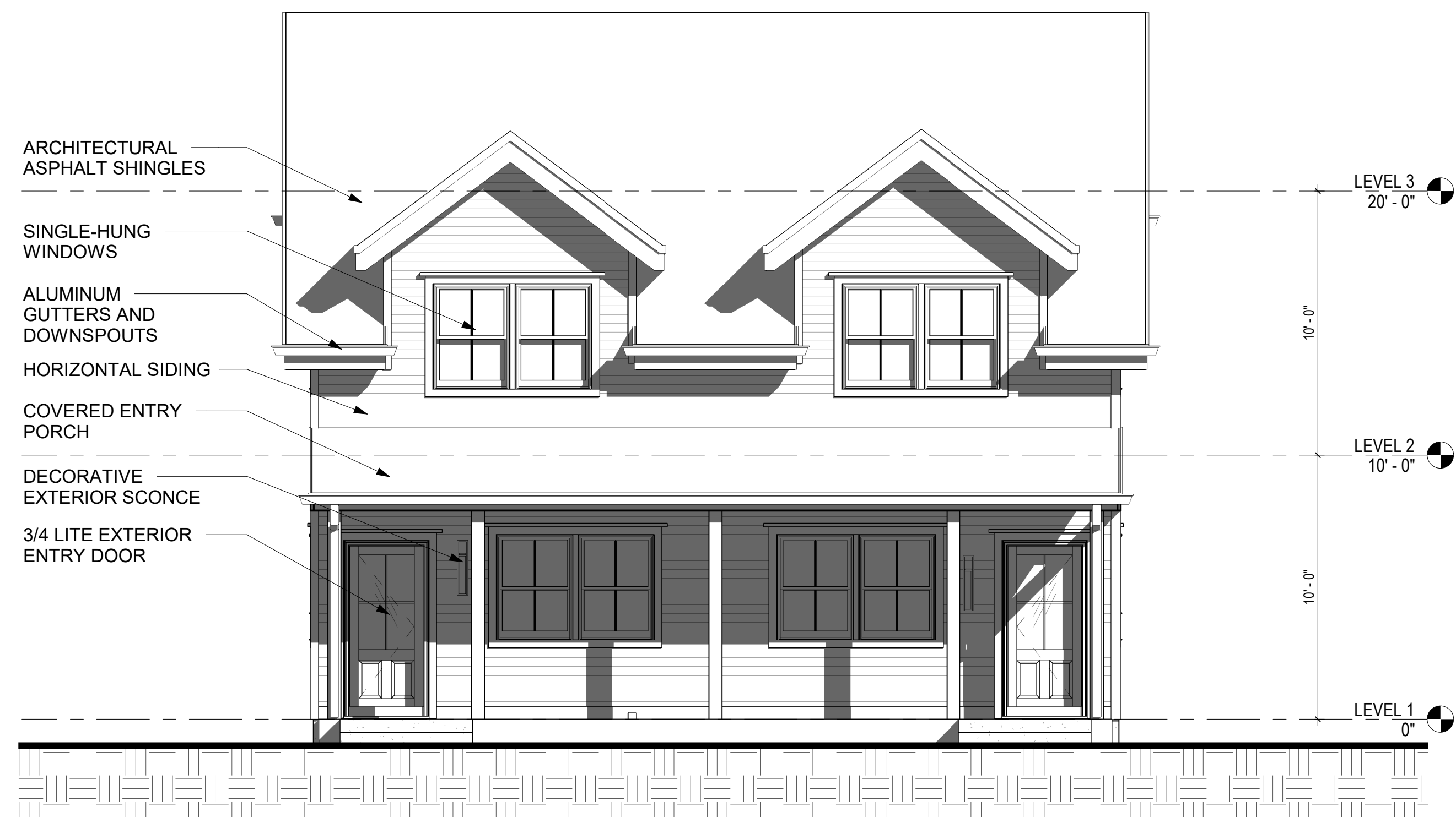
1 FRONT ELEVATION - BUILDING 1 & 3 A3.0A 1/4" = 1'-0"
