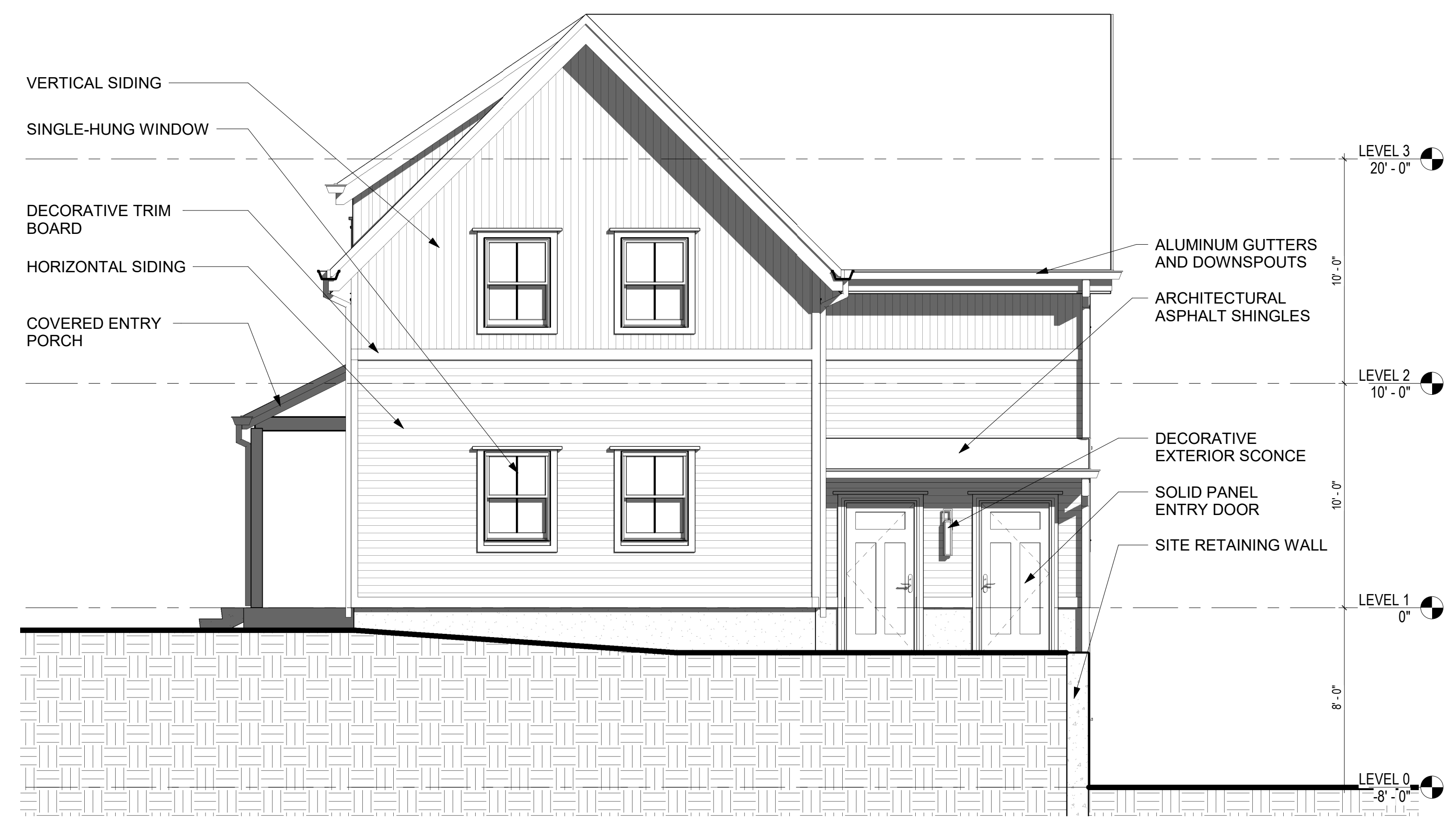
1 RIGHT ELEVATION - BUILDING 4 A3.1D 1/4" = 1'-0"
